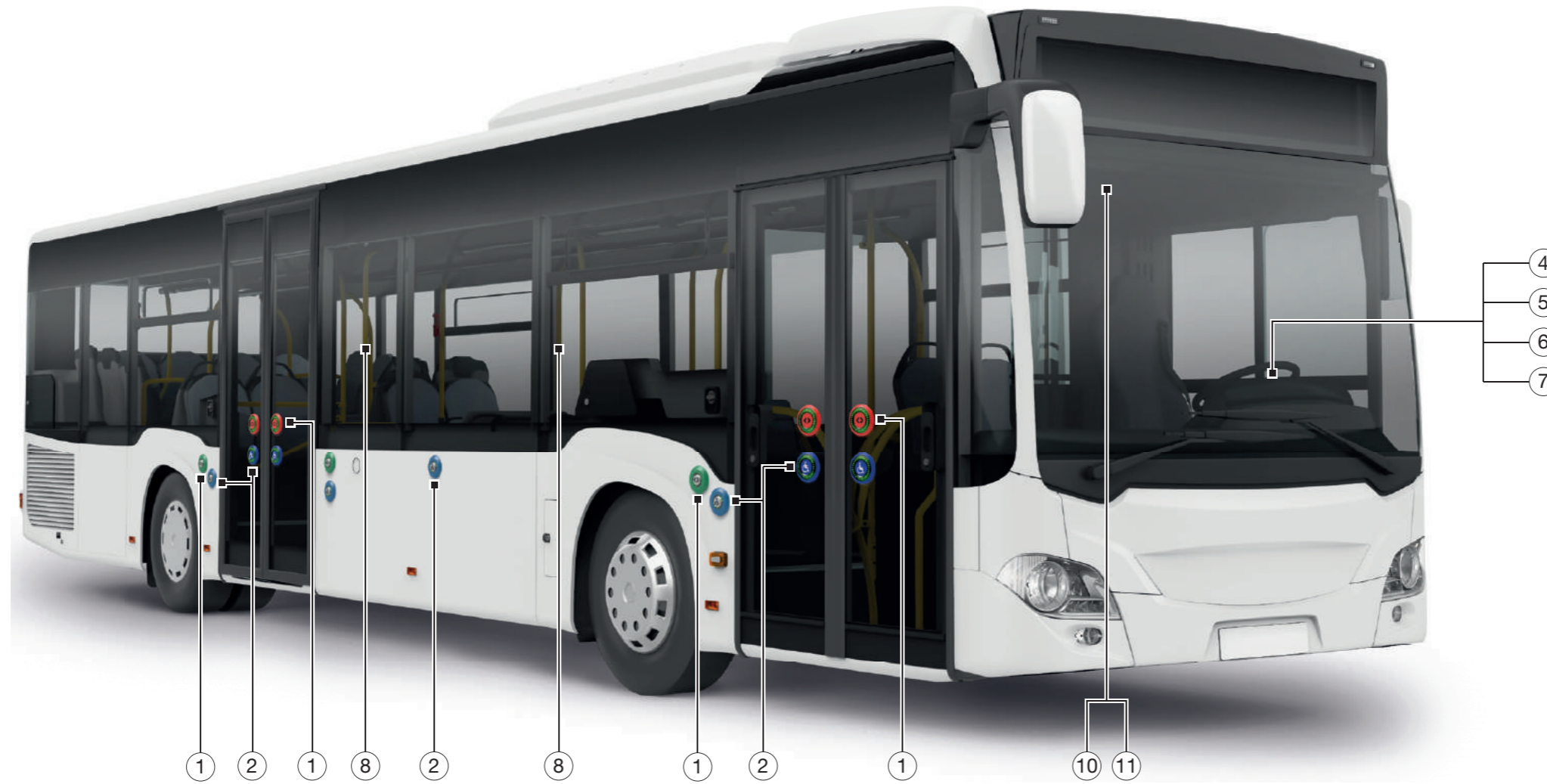
Typical HMI mounting locations on a bus (several positions per application shown).
